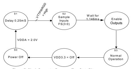
Figure 7. Clock Generator Power-up/Run State Diagram
