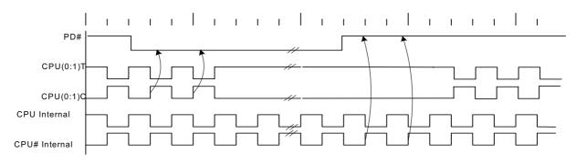
Figure 5. Power-down Assertion/Deassertion Timing Waveforms - Nonbuffered Mode
