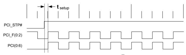
Figure 4. Deassertion PCI\_STP# Waveform<sup>[7]</sup>
