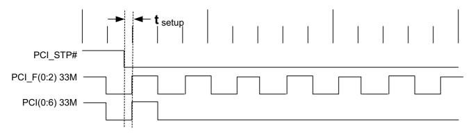
Figure 3. Assertion PCI\_STP# Waveform
