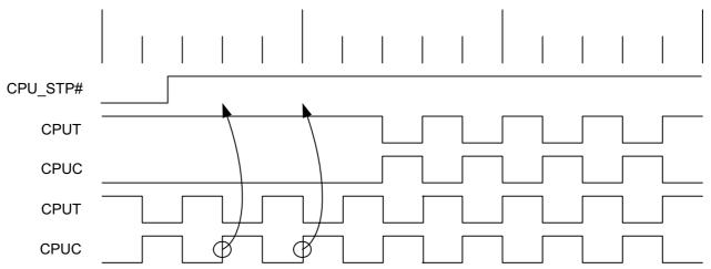
Figure 2. Deassertion CPU\_STP# Waveform
